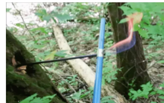
Flammable gas being emitted from increment borer at time of sampling.
